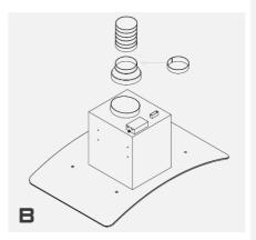
Hood Must Be Installed On Minimum 5" Round Ducting or Rectangular Equivalent
